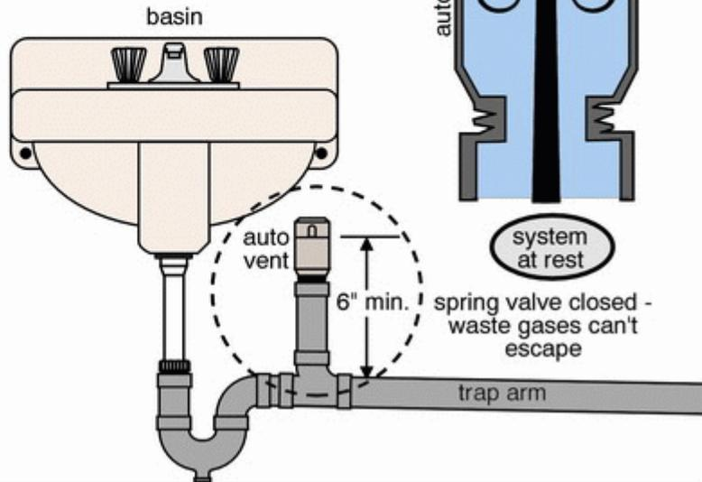
spring valve closed - waste gases can't escape
