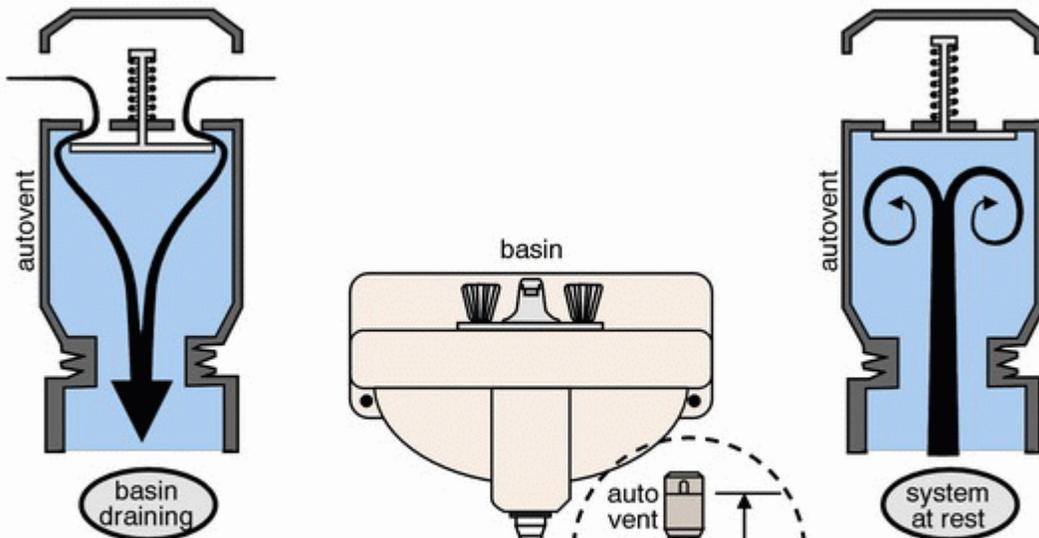
waste piping under negative pressure - spring valve opens to let air into the system
